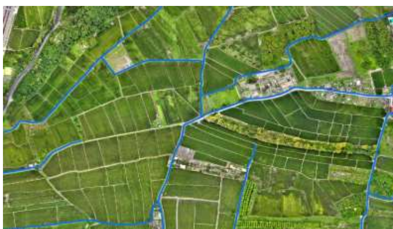
Figure 8. Orthoimage overlaid with canal map
