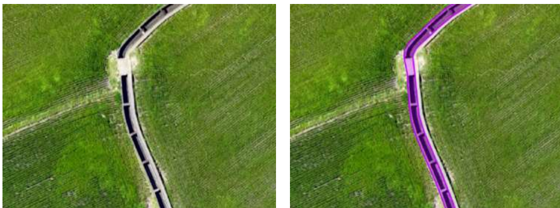
Figure 9. Polygon digitization results according to the actual width of the canal
