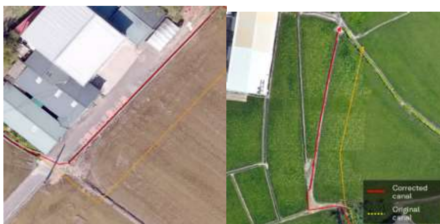
Figure 7. Canal map correction (error digitation on farm)
