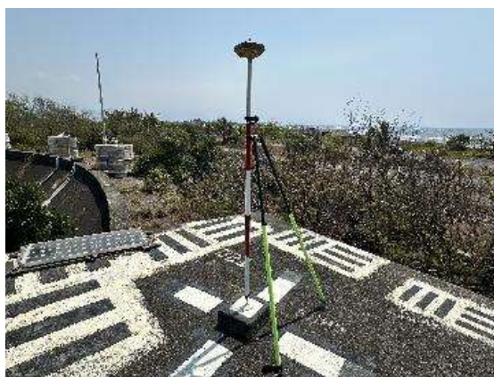
Figure 4. National control point surveying
