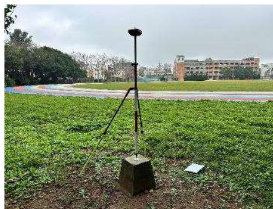
Figure 4. National control point surveying
